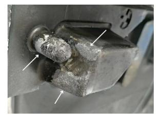
**Fig. 1** – Corroded die causing die soldering. The white arrows indicate the most worn regions.
