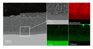
**Fig. 2** – SEM and EDS images of soldered aluminum on AISI H13 surface after 10 minutes of corrosion in molten aluminum (A383) at 720 °C.
